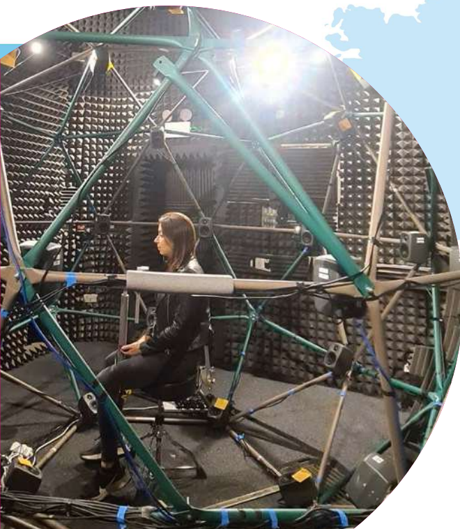
Below: Measurement of the Head Related Transfer Function (HRTF). Courtesy of the Turret Laboratory, Imperial College London, www.axdesign.ac.uk
